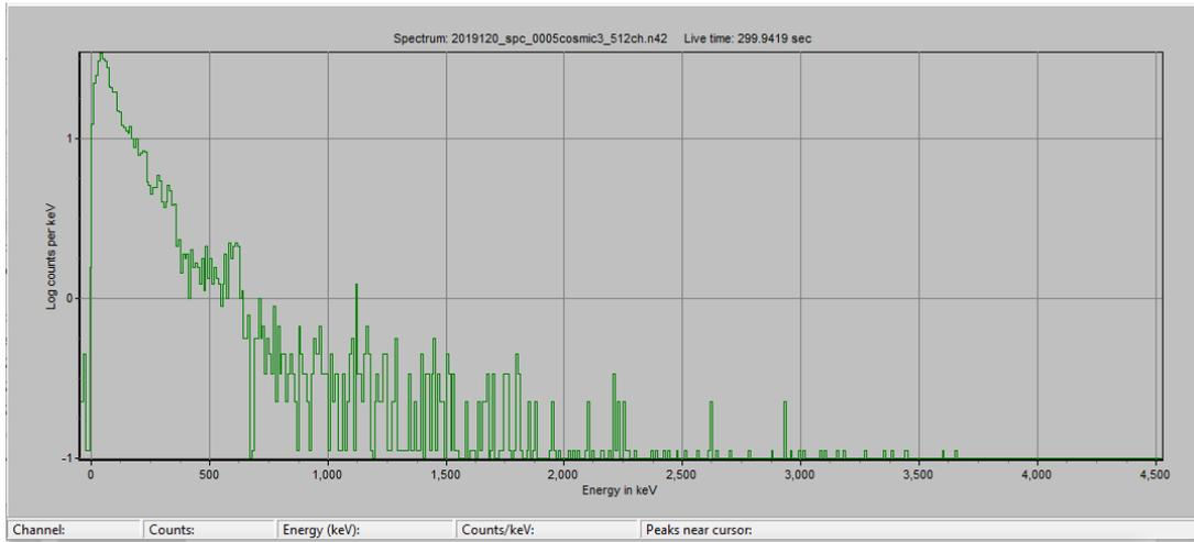
Figure 6. Spectrum acquired by a NaI 2''x2'' at Banyoles lake (Barcelona, Spain).
