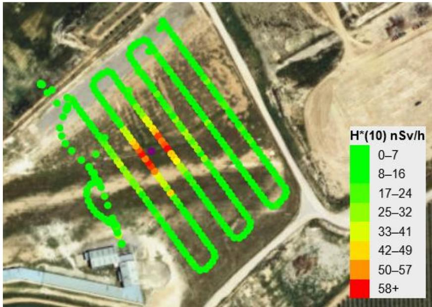
Figure 9.  $H^*(10)$  rate map of a 2''X2'' NaI detector mounted on a RWUAS, flying over a  $^{137}\text{Cs}$  point source of 346 MBq at 20 m altitude a.g.l. with a horizontal velocity of approximately  $3 \text{ m s}^{-1}$ . The calculated location of the source is indicated by a violet dot.
