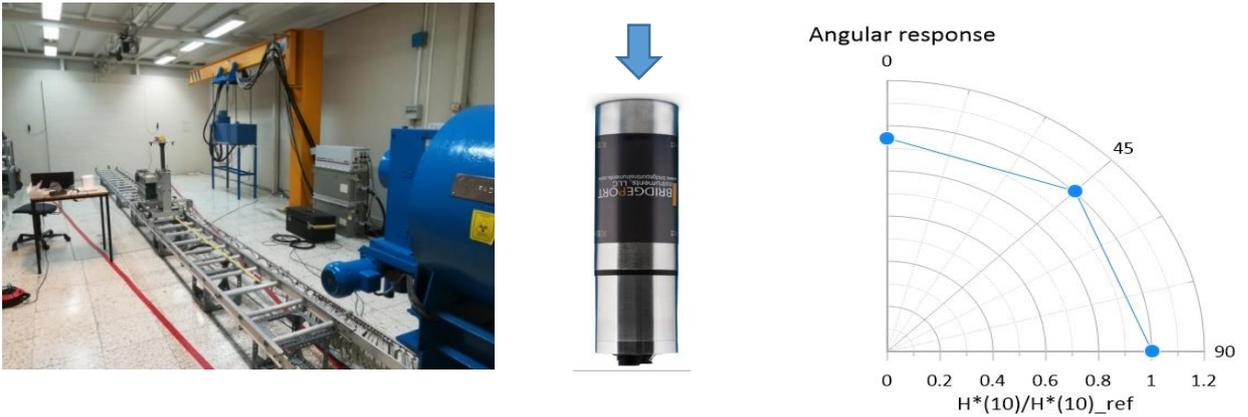
Figure 2. Experimental relative response of a NaI 2''x2'' scintillator at different angles and  $^{137}\text{Cs}$  source (90° incident gamma photons in the direction of the vertical axes of the detector)
