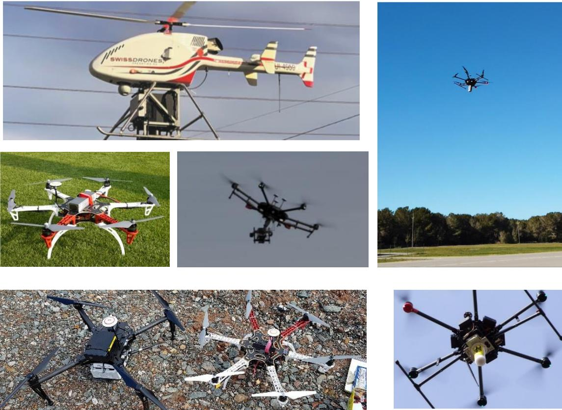
*Figure 1.* Top left: Huge SWISSDRONES SDO 50 drone with an HPGe detector; middle left: small DJI F550 with a CZT 1.5 cm<sup>3</sup> detector; top right: medium DJI Matrice 600 with a NaI 2"x2"; middle center: Medium DJI Matrice 600 UAS and gimbal with a "localizer detector" bottom left: DJI M100 with a 1"x1"x2" CsI (left) and the DJI F550 with a Geiger Muller (right) and bottom right: DJI Matrice 600 with a CeBr<sub>3</sub> 1.5"x1.5" detector.
