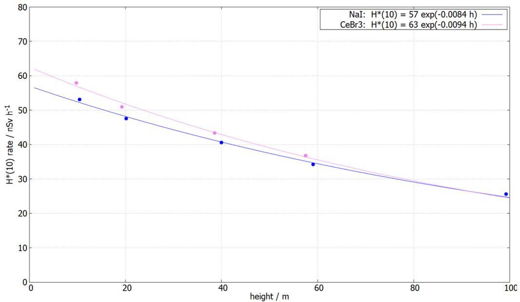
Figure 8.  $H^*(10)$  rate at different altitudes using the summed spectra. Exponential functions are fitted for the different scintillator detectors.
