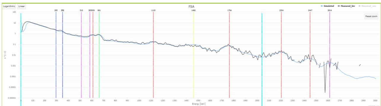
Figure 4. Measured count rate in former Uranium mines at Seelingstädt (Germany) and simulated spectra to determine the radionuclide activities using FSA. The altitude of the measurements was 20 m a.g.l., the speed of the drone  $2.8 \text{ m s}^{-1}$  and the spectrum the total integration time was 44 s.
