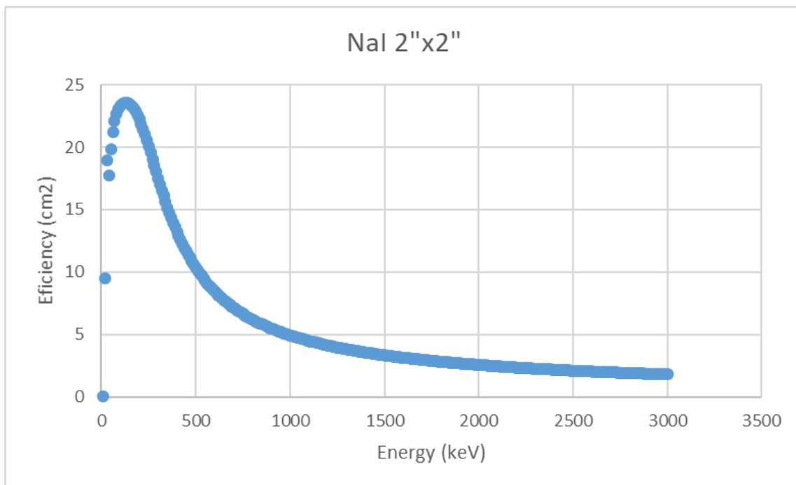
Figure 7. Efficiency per unit fluence rate obtained with Monte Carlo simulations for a NaI 2''x2'' expressed in cm<sup>2</sup>.
