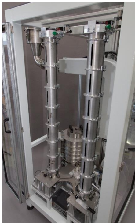
Stacks for stored filters
